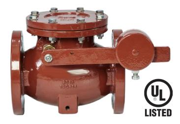
The Soval 826 Series Lever and Weight Swing Check Valves are manufactured to AWWA C508 Standard and are UL Listed designed for use in water and wastewater applications.
